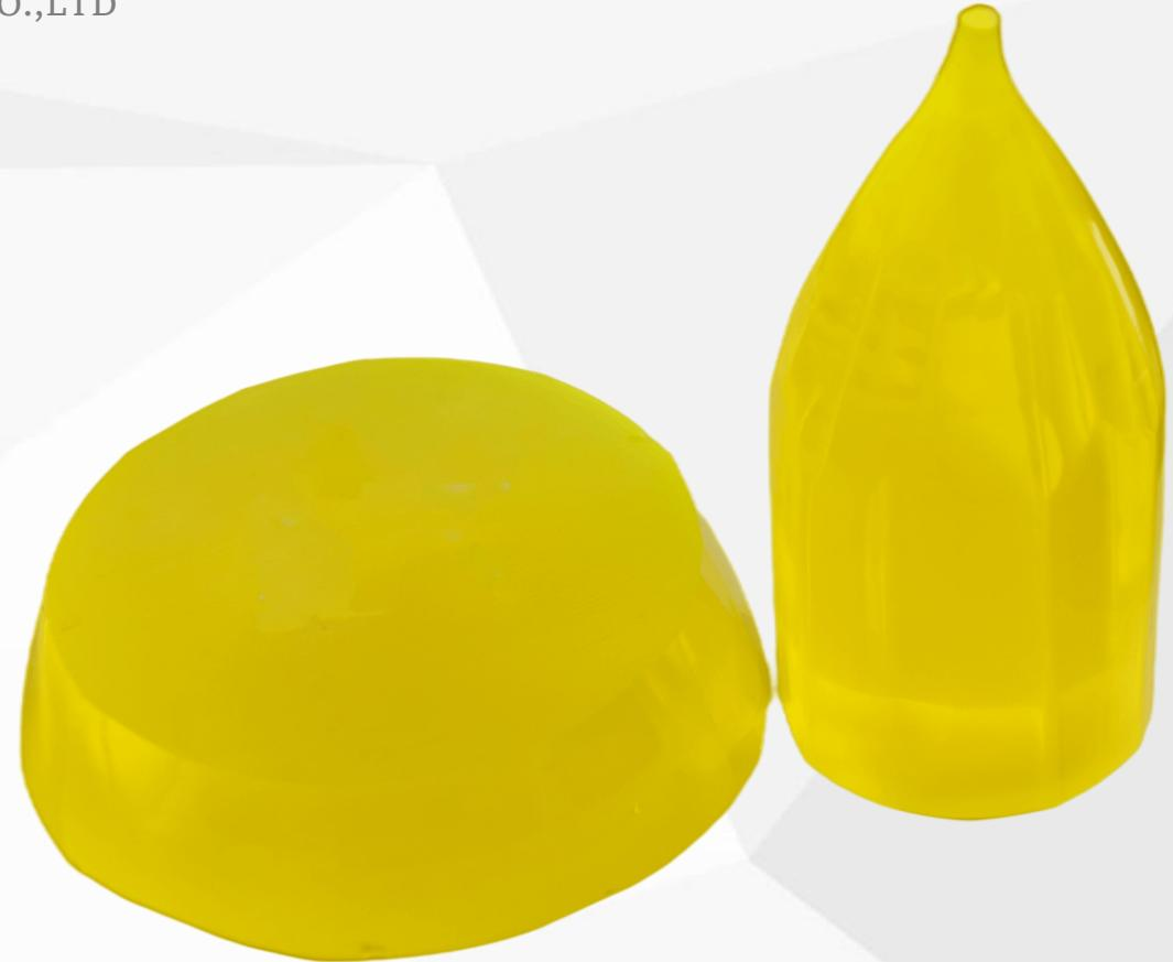
At this time, a high coupling efficiency can be achieved. Furthermore, Ce:YAG can also be commonly used as a phosphor in cathode ray tubes and white light-emitting diodes.
