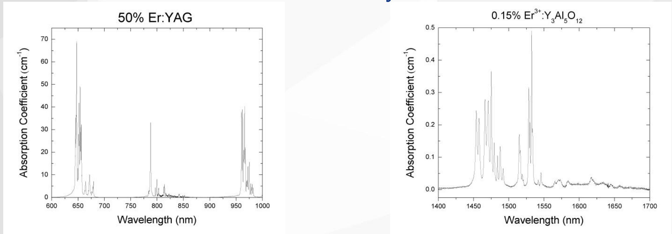
Absorption coefficient of with different Erbium ion doping
