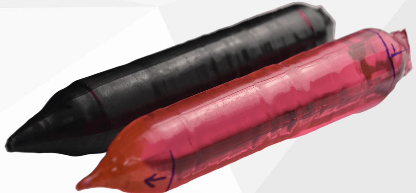
Er<sup>3+</sup>:YAG crystal is an attractive laser material for eye-safe emission at wavelengths of 1617 and 1645 nm which can be resonantly diode-pumped into the upper laser manifold at 1470 nm and 1532 nm.
