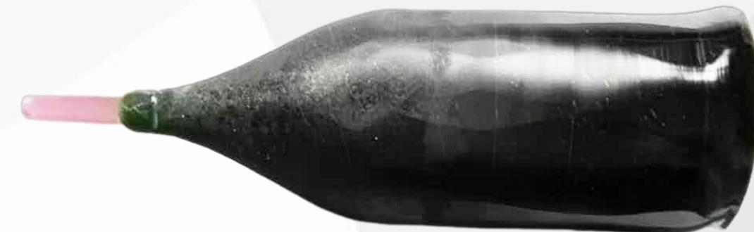
Active elements manufactured from YSGG crystals are optimum for medium power pulse lasers with the repetition rates of up to several tens of cycles. The advantages of YSGG crystals compared with YAG crystals are lost when large size elements are used because of the worse thermal characteristics of YSGG crystals.
