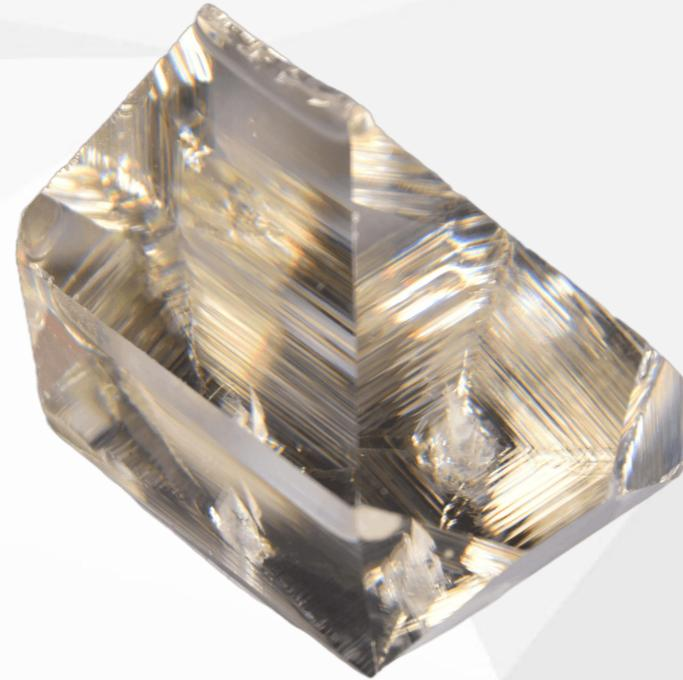
In addition to unique NLO features, KTP also has promising E-O and dielectric properties that are comparable to LiNbO<sub>3</sub>. These advantaged properties make KTP extremely useful to various E-O devices.
