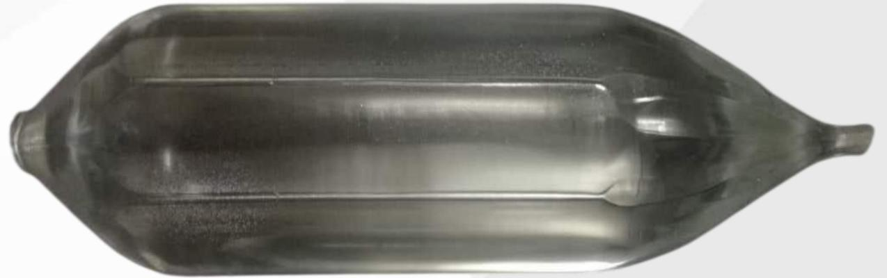
Undoped YAG Crystal or Pure yttrium aluminium garnet provides an interesting alternative to sapphire for UV optics, IR optics and refractometry
