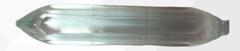
Yb:YAG shows great promise as a high power laser material. Several applications are being developed in the field of industrial lasers, such as metal cutting and welding. With high quality Yb:YAG now available, additional fields and applications are being explored.
